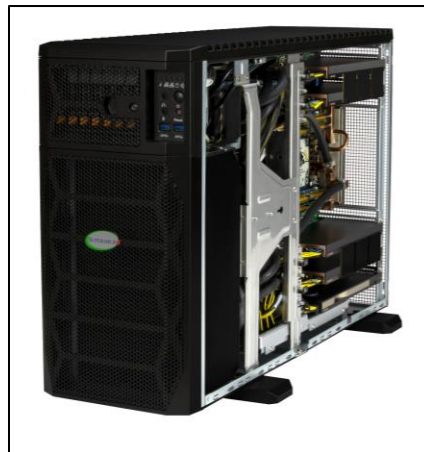
Figure 7 - Open Side View of Liquid Cooled System
