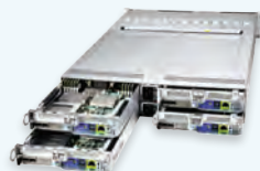
2U 4-Node BigTwin® (Liquid cooling option)
